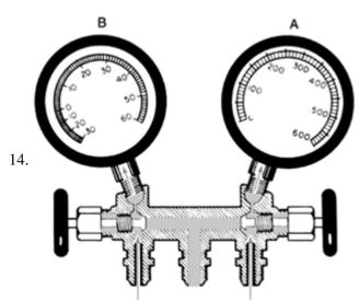
The tool in the figure above is being discussed. *Technician A* says the "B" gauge will register vacuum in Hg as well as psig. *Technician B* says the "A" gauge will register pressure in psig. Who is correct?
