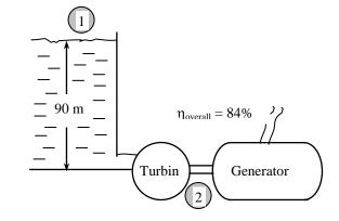
**2-123** An entrepreneur is to build a large reservoir above the lake level, and pump water from the lake to the reservoir at night using cheap power, and let the water flow from the reservoir back to the lake during the day, producing power. The potential revenue this system can generate per year is to be determined.
