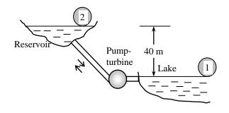
$$\dot{W}_{\text{max, turbine}} = \dot{W}_{\text{min, pump}} = \dot{W}_{\text{ideal}} = \Delta \dot{E}_{\text{mech}} = \dot{m}\Delta e_{\text{mech}} = \dot{m}\Delta p e = \dot{m}g\Delta z = \rho \dot{V}g\Delta z$$
