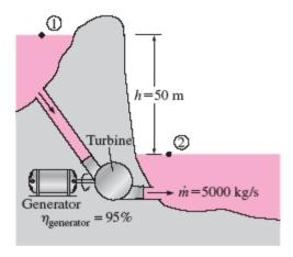
Then the rate at which mechanical energy of fluid supplied to the turbine and the overall efficiency become
