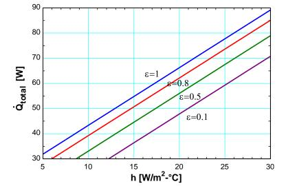
**2-101** A 1000-W iron is left on the iron board with its base exposed to the air at 23°C. The temperature of the base of the iron is to be determined in steady operation.
