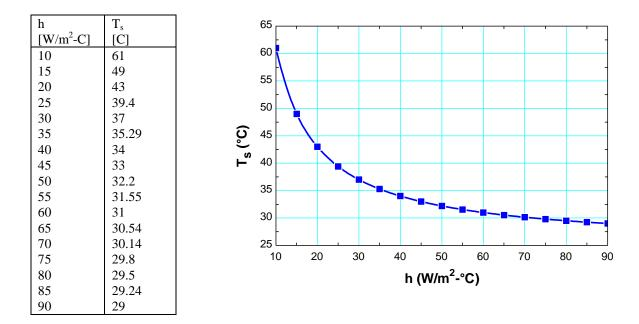
**2-105** A spacecraft in space absorbs solar radiation while losing heat to deep space by thermal radiation. The surface temperature of the spacecraft is to be determined when steady conditions are reached..
