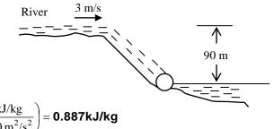
$$e_{\text{mech}} = pe + ke = gh + \frac{V^2}{2} = \left( (9.81 \,\text{m/s}^2)(90 \,\text{m}) + \frac{(3 \,\text{m/s})^2}{2} \right) \left( \frac{1 \,\text{kJ/kg}}{1000 \,\text{m}^2/\text{s}^2} \right) = 0.887 \,\text{kJ/kg}$$
