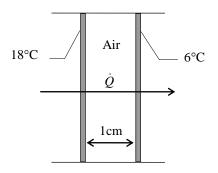
**2-96** Two surfaces of a flat plate are maintained at specified temperatures, and the rate of heat transfer through the plate is measured. The thermal conductivity of the plate material is to be determined.
