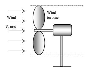
$$\dot{W}_{\text{max},1} = \dot{E}_{\text{mech},1} = \dot{m}_1 e_{\text{mech},1} = \rho V_1 A k e_1 = (1.25 \text{ kg/m}^3)(7 \text{ m/s})(1 \text{ m}^2)(0.0245 \text{ kJ/kg}) = 0.2144 \text{ kW}$$
