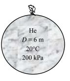
**3-78 EES** Problem 3-77 is to be reconsidered. The effect of the balloon diameter on the mass of helium contained in the balloon is to be determined for the pressures of (a) 100 kPa and (b) 200 kPa as the diameter varies from 5 m to 15 m. The mass of helium is to be plotted against the diameter for both cases.
