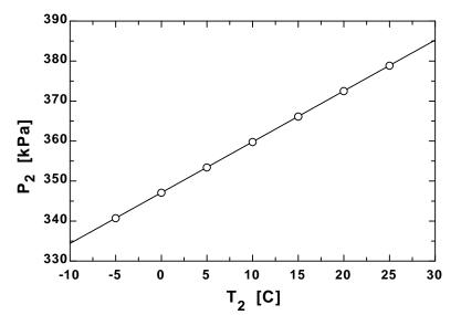
**3-129** A large tank contains nitrogen at a specified temperature and pressure. Now some nitrogen is allowed to escape, and the temperature and pressure of nitrogen drop to new values. The amount of nitrogen that has escaped is to be determined.
