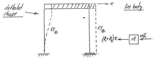
equation of motion:  $M\ddot{x} + kx = 0$  or  $\ddot{x} + \frac{k}{M}x = 0$  Als
