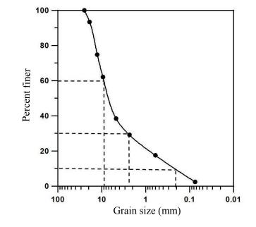
b. The grain-size distribution curve for the mixture is drawn below.
