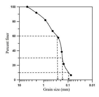
b.  $D_{60} = 0.28 \text{ mm}$ ;  $D_{30} = 0.17 \text{ mm}$ ;  $D_{10} = 0.095 \text{ mm}$
