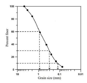
b.  $D_{10} = 0.13 \text{ mm}$ ;  $D_{30} = 0.3 \text{ mm}$ ;  $D_{60} = 0.9 \text{ mm}$
