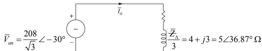
$$\bar{I}_a = \frac{\bar{V}_{an}}{(\bar{Z}_\Delta / 3)} = \frac{120.1\angle -30^\circ}{5\angle 36.87^\circ} = 24.02\angle -66.87^\circ \text{ A}$$
