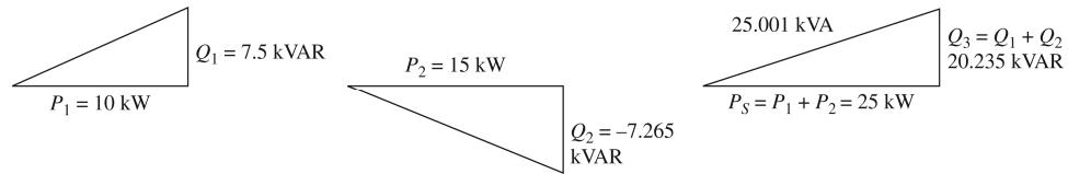
$$I_s = \frac{S_s}{\sqrt{3}V_{LL}} = \frac{25.001 \times 10^3}{\sqrt{3}(480)} = 30.07 \text{ A}$$
