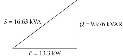
$$P_{3\phi} = \text{Re } \bar{S}_{3\phi} = 13.3 \text{ kW Delivered}$$
