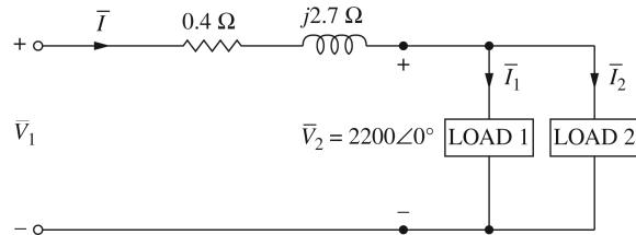
Phase voltage at the load terminals is  $V_2 = \frac{2200\sqrt{3}}{\sqrt{3}} = 2200 \text{ V}$  taken as Ref.
