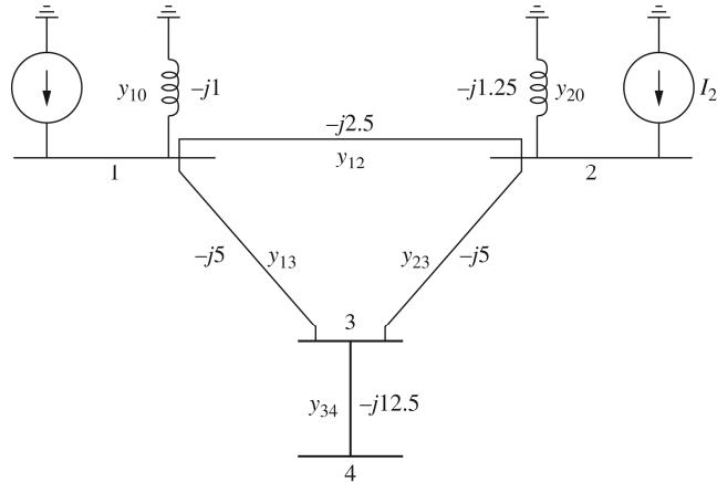
$$\bar{Y}_{BUS} = \begin{bmatrix} \bar{Y}_{11} & \bar{Y}_{12} & \bar{Y}_{13} & \bar{Y}_{14} \\ \bar{Y}_{21} & \bar{Y}_{22} & \bar{Y}_{23} & \bar{Y}_{24} \\ \bar{Y}_{31} & \bar{Y}_{32} & \bar{Y}_{33} & \bar{Y}_{34} \\ \bar{Y}_{41} & \bar{Y}_{42} & \bar{Y}_{43} & \bar{Y}_{44} \end{bmatrix} = j \begin{bmatrix} -8.5 & 2.5 & 5.0 & 0 \\ 2.5 & -8.75 & 5.0 & 0 \\ 5.0 & 5.0 & -22.5 & 12.5 \\ 0 & 0 & 12.5 & -12.5 \end{bmatrix} S$$
