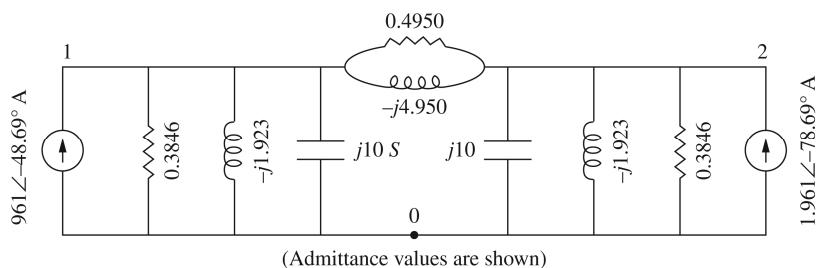
$$\left[ \begin{array}{c|c} (.3846 + j4.950) + j(10 - 1.923 - 4.950) & -(j4.950) \\ \hline -(j4.950) & (.3846 + j4.950) + j(10 - 1.923 - 4.950) \end{array} \right] \left[ \begin{array}{c} \bar{V}_{10} \\ \bar{V}_{20} \end{array} \right] = \left[ \begin{array}{c} 1.961\angle -48.69^\circ \\ 1.961\angle -78.69^\circ \end{array} \right]$$
