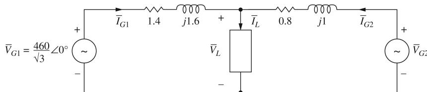
$$(a) \bar{I}_{G1} = \frac{15 \times 10^3}{\sqrt{8}(460)(0.8)} \angle -\cos^{-1} 0.8 = 23.53 \angle -36.87^\circ \text{ A}$$
