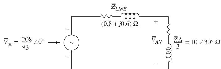
Using voltage division:  $\bar{V}_{AN} = \bar{V}_{an} \frac{\bar{Z}_\Delta / 3}{(\bar{Z}_\Delta / 3) + \bar{Z}_{LINE}}$
