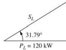
$$\begin{aligned}Q_L &= P_L \tan(31.79^\circ) \\ &= 74.364 \text{ kVAR}\end{aligned}$$
