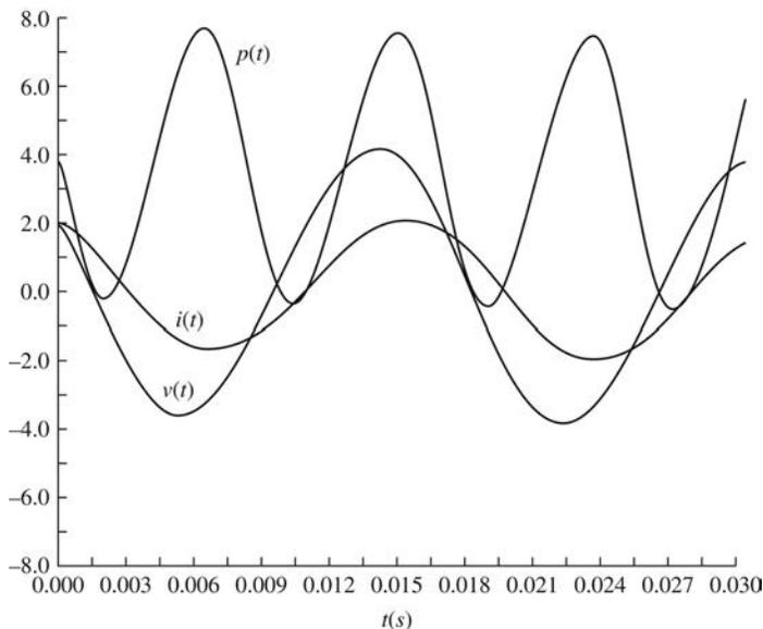
**2.16** (a)  $\bar{Z} = 10 + j120\pi \times 0.04 = 10 + j15.1 = 18.1 \angle 56.4^\circ \Omega$
