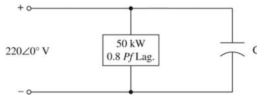
$$\begin{aligned}P_{old} &= 50 \text{ kW}; \cos^{-1} 0.8 = 36.87^\circ; \theta_{OLD} = 36.87^\circ; Q_{old} = P_{old} \tan(\theta_{old}) \\ &= 37.5 \text{ kVAR}\end{aligned}$$
