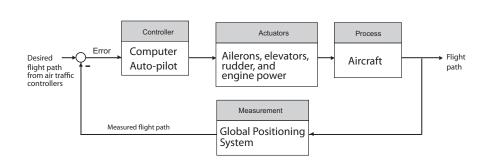
An aircraft flight path control system using GPS:
