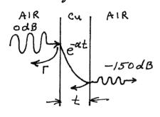
$$8_{s} = \sqrt{\frac{2}{\omega_{M}\sigma}} = 2.09 \times 10^{-6} \text{m} = \frac{1}{\alpha}$$
