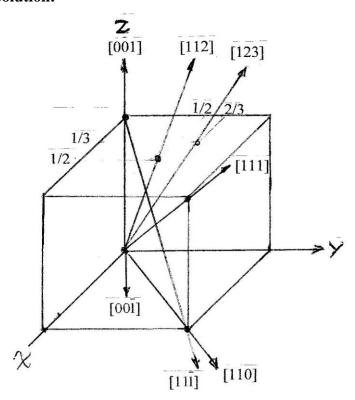
**Problem 2.14:** (a) Compare the linear atom density of the [100] and [111] directions in the BCC metal iron, with a lattice parameter of 0.286 nm. (b) Which is the most closely packed direction in the BCC structure? (c) What is the radius of an iron atom if it is assumed that the atoms touch along the most closely packed direction?
