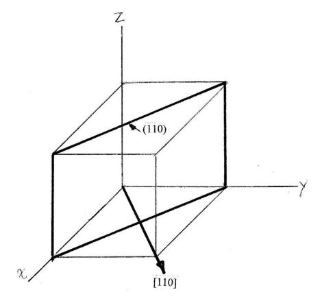
(c) Starting at the position 0, 0, 0 and going to the position 1, 1, 0 the [110] direction is sliced into two segments. There is a (110) plane that surrounds the atoms both at 0, 0, 0 and at 1, 1, 0. The distance from 0, 0, 0 to 1, 1, 0 is  $a2^{1/2}$ , but the spacing between planes is 1/2 of this value, because the (111) planes cut this distance into two segments. Thus the spacing between the (110) planes is
