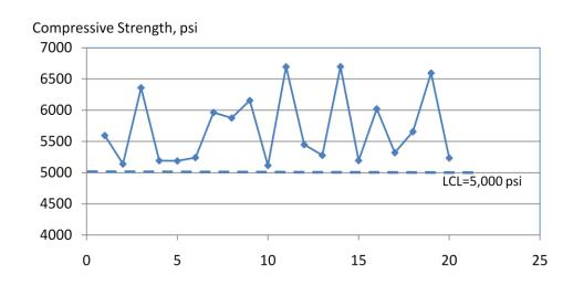
The target value is any value above the specification limit of 5,000 psi. The plant production is meeting the specification requirement.
