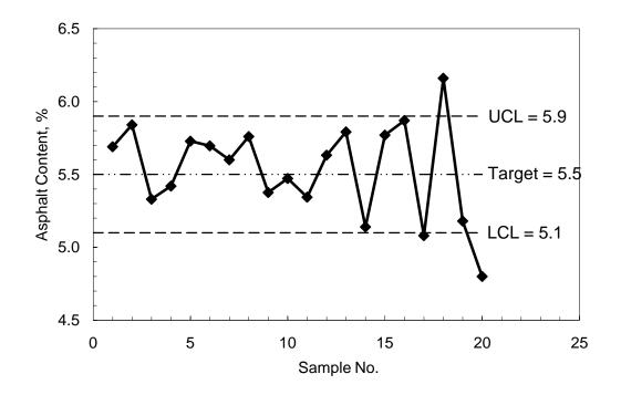
The control chart shows that most of the samples have asphalt content within the specification limits. Only few samples are outside the limits. The plot shows no specific trend, but large variability especially in the last several samples.
