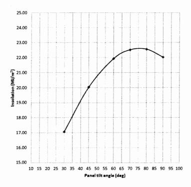
As shown in the graph, the insolation corresponding to this tilt angle is
