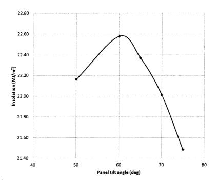
As shown in the graph, the optimum tilt angle is approximately  $61^{\circ}$ , but this angle is measured with respect to the horizontal. The roof has a 4 on 12 pitch, which means that the angle of the roof with respect to the horizontal is  $\tan^{-1}(4/12) = 18.4^{\circ}$ . Thus, the optimum angle of the solar panel with respect to the roof is
