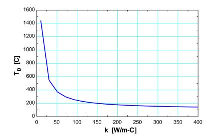
**2-103** A spherical communication satellite orbiting in space absorbs solar radiation while losing heat to deep space by thermal radiation. The heat generation rate and the surface temperature of the satellite are to be determined.
