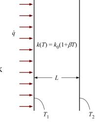
**2-112** A plate with variable conductivity is subjected to specified temperatures on both sides. The rate of heat transfer through the plate is to be determined.
