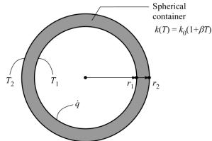
**2-118** A spherical shell with variable conductivity is subjected to specified temperatures on both sides. The variation of temperature and the rate of heat transfer through the shell are to be determined.
