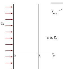
**2-139E** A large plane wall is subjected to a specified temperature on the left (inner) surface and solar radiation and heat loss by radiation to space on the right (outer) surface. The temperature of the right surface of the wall and the rate of heat transfer are to be determined when steady operating conditions are reached.
