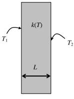
Then the rate of heat conduction through the plate becomes
