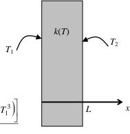
2-113 The thermal conductivity of stainless steel has been characterized experimentally to vary with temperature. The average thermal conductivity over a given temperature range and the  $k(T) = k_0 (1 + \beta T)$  expression are to be determined. Assumptions 1 Thermal conductivity varies with temperature.
