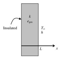
**2-87E** Heat is generated in a large plane wall whose one side is insulated while the other side is maintained at a specified temperature. The mathematical formulation, the variation of temperature in the wall, and the highest temperature in the wall are to be determined for steady one-dimensional heat transfer.
