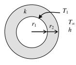
2-75 Pro A spherical container is used for storing chemicals undergoing exothermic reaction that provides a uniform heat flux to its inner surface. The outer surface is subjected to convection heat transfer. The variation of temperature in the container wall and the inner and outer surface temperatures are to be determined for steady one-dimensional heat transfer.
