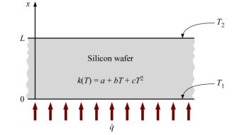
The maximum allowable heat flux such that the temperature difference across the wafer thickness does not exceeding 2 °C is
