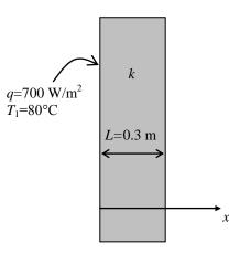
**2-58** The base plate of a household iron is subjected to specified heat flux on the left surface and to specified temperature on the right surface. The mathematical formulation, the variation of temperature in the plate, and the inner surface temperature are to be determined for steady one-dimensional heat transfer.
