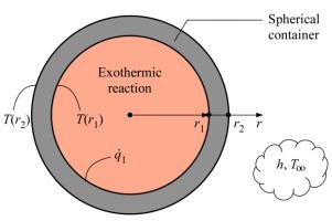
**2-76** A spherical container is subjected to uniform heat flux on the outer surface and specified temperature on the inner surface. The mathematical formulation, the variation of temperature in the pipe, and the outer surface temperature, and the maximum rate of hot water supply are to be determined for steady one-dimensional heat transfer.
