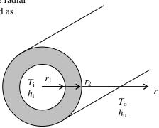
**2-146** A 10-m tall exhaust stack discharging exhaust gases at a rate of 1.2 kg/s is subjected to solar radiation and convection at the outer surface. The variation of temperature in the exhaust stack and the inner surface temperature of the exhaust stack are to be determined.
