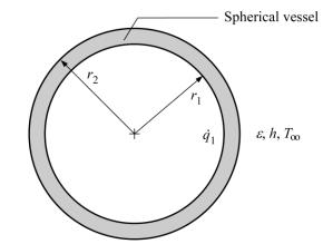
**2-142** A small hot metal object is allowed to cool in an environment by convection. The differential equation that describes the variation of temperature of the ball with time is to be derived.
