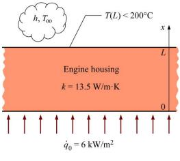
**2-62** A plane wall is subjected to uniform heat flux on the left surface, while the right surface is subjected to convection and radiation heat transfer. The variation of temperature in the wall and the left surface temperature are to be determined for steady one-dimensional heat transfer.
