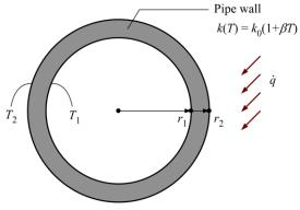
**2-115** A pipe is used for transporting boiling water with a known inner surface temperature in surroundings of cooler ambient temperature and known convection heat transfer coefficient. The pipe wall has a variable thermal conductivity. The outer surface temperature of the pipe is to be determined to ensure that it is below 50°C.
