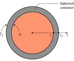
**2-73** A spherical shell is subjected to uniform heat flux on the inner surface, while the outer surface is subjected to convection heat transfer. The variation of temperature in the shell wall and the outer surface temperature are to be determined for steady one-dimensional heat transfer.
