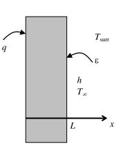
**2-144** A large plane wall is subjected to convection on the inner and outer surfaces. The mathematical formulation, the variation of temperature, and the temperatures at the inner and outer surfaces to be determined for steady one-dimensional heat transfer.
