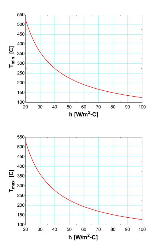
**2-85** Both sides of a large stainless steel plate in which heat is generated uniformly are exposed to convection with the environment. The location and values of the highest and the lowest temperatures in the plate are to be determined.
