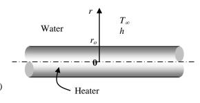
**2-98** A long resistance heater wire is subjected to convection at its outer surface. The surface temperature of the wire is to be determined using the applicable relations directly and by solving the applicable differential equation.
