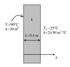
**2-60** A large plane wall is subjected to convection on the inner and outer surfaces. The mathematical formulation, the variation of temperature, and the temperatures at the inner and outer surfaces to be determined for steady one-dimensional heat transfer.
