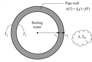
A pipe is used for transporting hot fluid with a known inner surface temperature. The pipe wall has a variable 2-116 thermal conductivity. The pipe's outer surface is subjected to radiation and convection heat transfer. The outer surface temperature of the pipe is to be determined.
