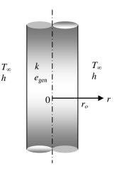
**2-99** A long homogeneous resistance heater wire with specified surface temperature is used to heat the air. The temperature of the wire 3.5 mm from the center is to be determined in steady operation.
