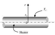
**2-92** A 2-kW resistance heater wire with a specified surface temperature is used to boil water. The center temperature of the wire is to be determined.
