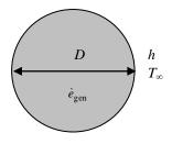
**2-152** A spherical reactor of 5-cm diameter operating at steady condition has its heat generation suddenly set to 9  $MW/m^3$ . The time rate of temperature change in the reactor is to be determined.
