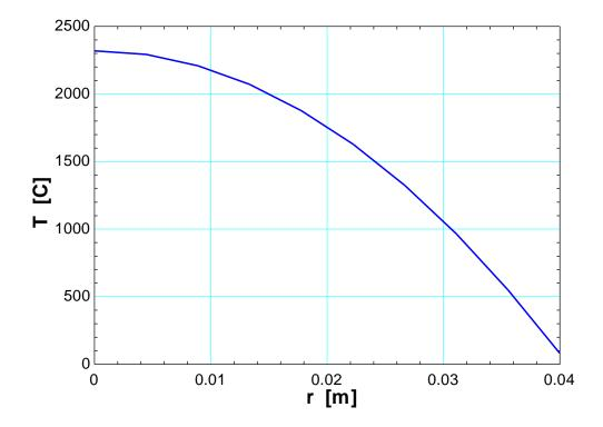
**2-95** A cylindrical nuclear fuel rod is cooled by water flowing through its encased concentric tube. The average temperature of the cooling water is to be determined.
