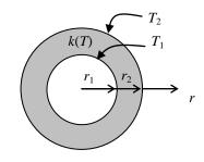
2-119 A spherical vessel, filled with chemicals undergoing an exothermic reaction, has a known inner surface temperature. The wall of the vessel has a variable thermal conductivity. Convection heat transfer occurs on the outer surface of the vessel. The minimum wall thickness of the vessel is to be determined so that the outer surface temperature is 50°C or lower.
