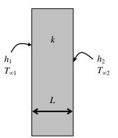
**2-61** Pro An engine housing (plane wall) is subjected to a uniform heat flux on the inner surface, while the outer surface is subjected to convection heat transfer. The variation of temperature in the engine housing and the temperatures of the inner and outer surfaces are to be determined for steady one-dimensional heat transfer.
