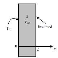
2-88 Heat is generated in a large plane wall whose one side is insulated while the other side is maintained at a specified temperature. The mathematical formulation, the variation of temperature in the wall, and the temperature of the insulated surface are to be determined for steady one-dimensional heat transfer.
