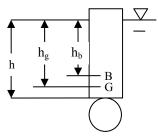
$$(Vol_s)(SG_s)(\gamma) + (Vol_p)(SG_p)(\gamma) = (Vol_s)(\gamma) + (Vol_p)(\gamma)$$
