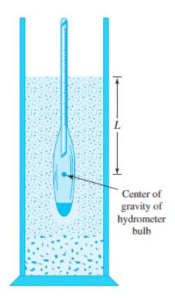
The larger grains would have settled beyond the zone of measurement. Hydrometers are designed to give the amount of soil, in grams, that is still in suspension.
