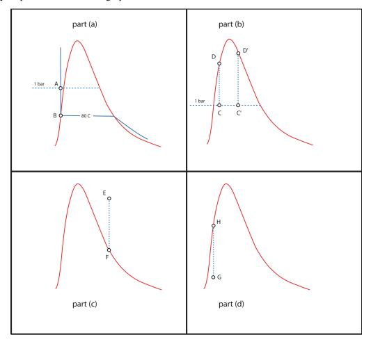
a) The initial state (A) is compressed liquid (80 °C, 1.013 bar). The process is conducted under constant volume. Assuming the isotherm to be vertical, the final state, B, is at the same temperature *and* on the saturation line. Therefore: T = 80 °C, P = 47.36 kPa.
