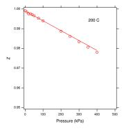
The line shown is tangent to the points at P = 0 and its slope is  $-5.00554 \times 10^{-5}$ . The easy way to draw this line is to fit a straight line through the points closest to the origin, say below 200 kPa. A smarter way is to use all the points and a *quadratic* equation:
