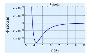
a) The potential has a minimum just above 4 Å or so. To determine this value accurately we must set the derivative of the potential equal to zero solve for the value of r. To do this easily, we define a new variable  $x = r/\sigma$  and rewrite the potential as:
