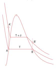
Both sides of the tank undergo constant-volume processes as indicated by the dashed lines. The graph shows the two states at the initial temperature T, as well as the states at some higher temperature,  $T + \delta$ . It is obvious that the pressure in the liquid side will always be *higher* than the pressure of the vapor side. Therefore, the pressure of 40 bar will be reached first in the liquid side, causing that alarm to go off.
