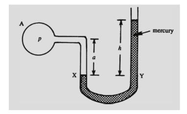
**Solution 1.9.** Start by equating the pressures at *X* and *Y*.
