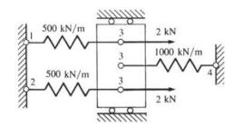
$$[k^{(1)}] = \begin{bmatrix} 500 & -500 \\ -500 & 500 \end{bmatrix}; [k^{(2)}] = \begin{bmatrix} 500 & -500 \\ -500 & 500 \end{bmatrix}; [k^{(3)}] = \begin{bmatrix} 1000 & -1000 \\ -1000 & 1000 \end{bmatrix}$$
