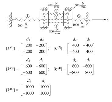
Assembling global [K] using direct stiffness method
