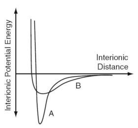
The well of titanium, represented by A, is deeper (higher melting point), has a larger radius of curvature (stiffer), and is more symmetric (smaller thermal expansion coefficient) than the well of aluminum, represented by B.
