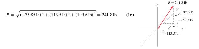
Write an expression for each force using Cartesian representation, and evaluate the resultant force vector. Sketch the resultant force in the xyz coordinate system.
