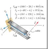
Determine the scalar and vector components of  $\vec{F}$  in direction  $\vec{r}_{AB}$ .
