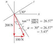
The t and n components are needed to determine if the box will slide using Coulomb's law of friction.
