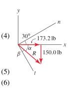
Alternate solution  $R_t$  and  $R_n$  may be determined using vector transformation concepts. Using Eqs. (2) and (3) described in Prob. 2.55, with  $\phi = -60^\circ$ , we obtain
