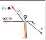
The mast of a ship supports forces from three cables as shown. If  $\alpha = 0^{\circ}$ , determine the value of *F* that will make the magnitude of the resultant of the three forces smallest.
