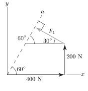
Note that  $\alpha$  equals 60° since  $F_1$  is perpendicular to line *a*. Using Cartesian representation,  $\vec{F}_1$  is given by
