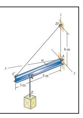
A wall-mounted jib crane consists of an I beam that is supported by a pin at point A and a cable at point C, where A and C lie in the xy plane. A crate at E is supported by a cable that is attached to a trolley at point B where the trolley may move along the length of the I beam. The forces supported by cables CD and BE are 3 kN and 5 kN, respectively. For the value of angle  $\alpha$  given below, determine expressions for the forces the two cables apply to the I beam.  $\alpha = 40^{\circ}$ .
