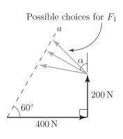
To determine the value of  $F_1$ , consider the sketch shown at the right. Noting that the hypotenuse of the upper triangle is given by
