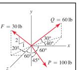
Write an expression for each force using Cartesian representation, and evaluate the resultant force vector. Sketch the resultant force in the xyz coordinate system.
