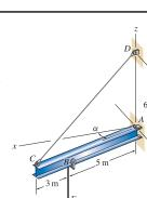
A wall-mounted jib crane consists of an I beam that is supported by a pin at point A and a cable at point C, where A and C lie in the xy plane. A crate at E is supported by a cable that is attached to a trolley at point B where the trolley may move along the length of the I beam. The forces supported by cables CD and BE are 3 kN and 5 kN, respectively. For the value of angle  $\alpha$  given below, determine expressions for the forces the two cables apply to the I beam.  $\alpha = 70^{\circ}$ .
