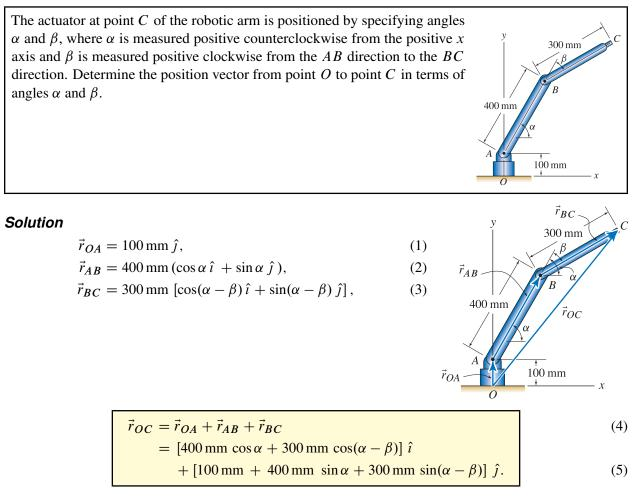
Some simple checks may be performed to help verify the accuracy of  $\vec{r}_{OC}$ , as follows
