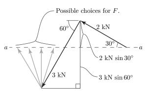
The magnitude of  $\vec{F}$  is then found by using the force polygon to write
