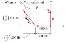
By examining the force polygon, the resultant force  $\vec{R}$  has the smallest magnitude when its direction is perpendicular to  $\vec{F}$ . For this situation, the *x* component of Eq. (1) is zero, which corresponds to
