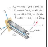
Determine the scalar and vector components of  $\vec{F}$  in direction  $\vec{r}_1$ .
