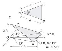
For the description and figure indicated below, determine the components of the cord force in directions parallel and perpendicular to rod CD. If released from rest, will the cord force tend to make bead E slide toward C or D?
