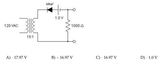
10) What is the minimum output voltage for this clipping circuit when the diode is not conducting?
