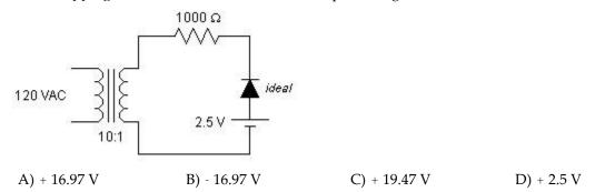
9) For this clipping circuit, what is the minimum output voltage when the diode is conducting?
