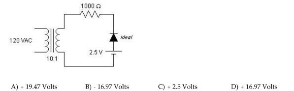
8) For this clipping circuit, what is the maximum output voltage when the diode is not conducting? 8) \_\_\_\_\_
