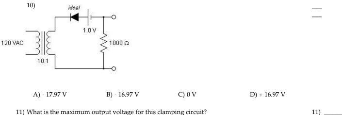
11) What is the maximum output voltage for this clamping circuit?
