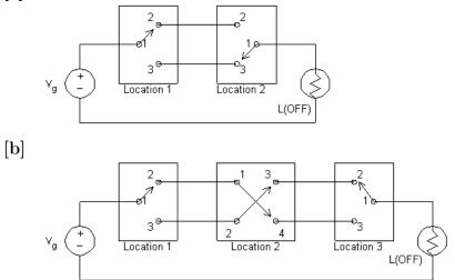
P 2.41 Each radiator is modeled as a  $48\,\Omega$  resistor:
