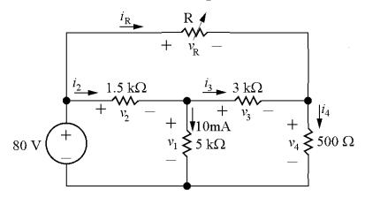
Ohms' law for 5 k $\Omega$  resistor:  $v_1 = (0.01)(5000) = 50$  V KVL for lower left loop:  $-80 + v_2 + 50 = 0 \rightarrow v_2 = 80 - 50 = 30$  V Ohm's law for 1.5 k $\Omega$  resistor:  $i_2 = v_2/1500 = 30/1500 = 20$  mA KCL at center node:  $i_2 = i_3 + 0.01 \rightarrow i_3 = i_2 - 0.01 = 0.02 - 0.01 = 0.01 = 10$  mA Ohm's law for 3 k $\Omega$  resistor  $v_3 = 3000i_3 = 3000(0.01) = 30$  V KVL for lower right loop:  $-v_1 + v_3 + v_4 = 0 \rightarrow v_4 = v_1 - v_3 = 50 - 30 = 20$  V
