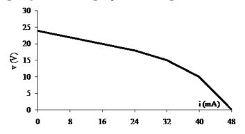
[b] Since the plot is linear for  $0 \le i_s \le 24$  mA and since  $R = \Delta v / \Delta i$ , we can calculate R from the plotted values as follows:
