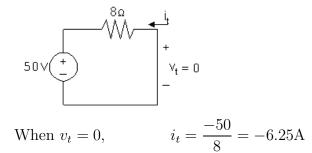
Note that this result can also be obtained by extrapolating the v - i characteristic to  $v_t = 0$ .
