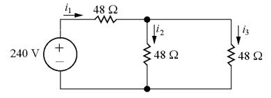
Write a KVL equation for the left and right loops:
