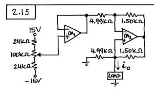
OA, provides a variable voltage from -10V to +10V, which OA, converts to a variable current from -2mA to +2mA.
