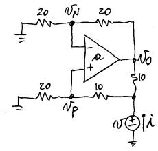
$$\nabla_{p} = \frac{2}{3} \nabla, \quad \nabla_{N} = \frac{1}{2} \nabla_{0}, \quad \nabla_{\theta} = \mathcal{A} \left( \nabla_{p} - \nabla_{N} \right) \\
