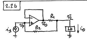
$V_{P} = V_{L} + R_{2}i_{S}$ ;  $V_{0} = A(V_{P} - V_{0}) \Rightarrow V_{0} = \frac{a}{Ha}V_{P}$   $V_{0} = \frac{a}{Ha}(V_{L} + R_{2}i_{S})$ .  $i_{0} = i_{S} + \frac{V_{0} - V_{L}}{R_{1}} \Rightarrow$   $i_{0} = i_{S} + \frac{1}{R_{1}}[\frac{a}{Ha}V_{L} - V_{L} + \frac{a}{Ha}R_{2}i_{S}] = Ai_{S} - \frac{1}{R_{0}}V_{L}$ ,  $A = 1 + (R_{2}/R_{1})/(1+1/a)$ ,  $R_{0} = R_{1}(1+a)$ .
