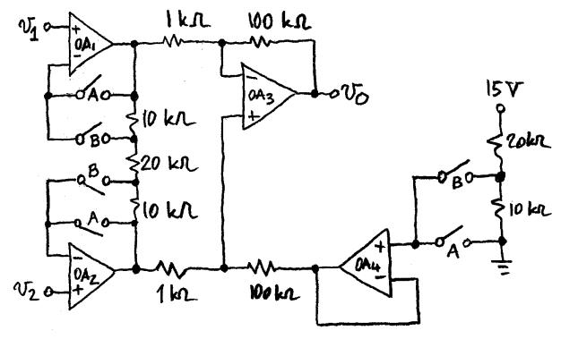
"A" switches closed  $\Rightarrow$   $V_0 = 1 \times 100 (V_2 - V_1) + 0 \text{ V}.$ "B" switches closed  $\Rightarrow$   $V_0 = (1 + 2\frac{10}{20}) \times 100 (V_2 - V_1) + 5 \text{ V}.$
