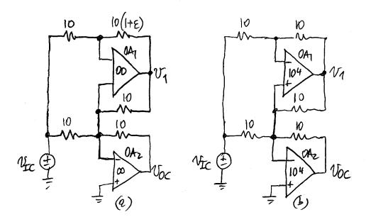
(a) Superposition:  $N_{OC} = -\frac{10}{10} V_{IC} - \frac{10}{10} V_{I}$ ,  $N_{I} = -\frac{10(1+\epsilon)}{10} N_{IC}$ :  $N_{OC} = -N_{I} + (1+\epsilon) V_{IC} = E N_{IC} \Rightarrow A_{CM} = E = 4 \frac{P}{100} = 4 \frac{0.1}{100} = \frac{1}{250} V_{N}$ .  $CMRR = 20 log 1/(1/250) \approx 48 dB$
