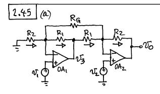
$v_{M} = v_{p_1} = v_1$ ,  $v_{N2} = v_{p_2} = v_2$ . Applying KCL:  $\frac{O-v_1}{R_2} = \frac{v_1-v_2}{R_6} + \frac{v_1-v_3}{R_1}$ ;  $\frac{v_2-v_0}{R_2} = \frac{v_1-v_2}{R_6} + \frac{v_3-v_2}{R_1}$ . Adding the two equations pairwise gives  $\frac{v_2-v_1}{R_2} - \frac{v_0}{R_2} = 2\frac{v_1-v_2}{R_6} + \frac{v_1-v_2}{R_1}$ . Solving for  $v_0 = (1 + \frac{R_2}{R_1} + 2\frac{R_2}{R_6})(v_2-v_1)$ .
