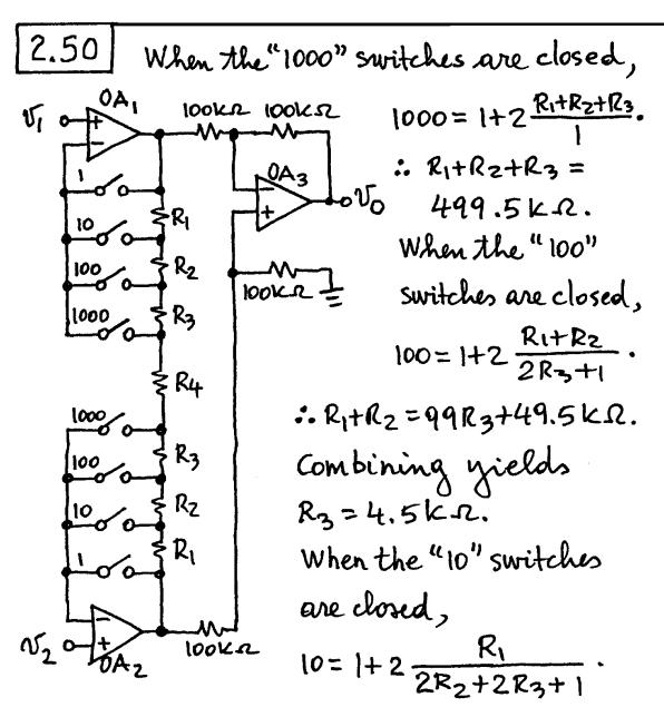
:.  $R_1 = 9R_2 + 45k\Omega$ . Combining yields  $R_2 = 45k\Omega$  and  $R_1 = 450k\Omega$ . Summarizing,  $R_1 = 450k\Omega$ ,  $R_2 = 45k\Omega$ ,  $R_3 = 4.5k\Omega$ ,  $R_4 = 1k\Omega$ . All other resistors = 100 k $\Omega$ .
