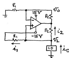
Use  $R_2 = 2.00 \text{ k/L}, 1\%$ . Then,  $V_0 = (1+2/10)V_L$ = 1.2  $V_L$ .
