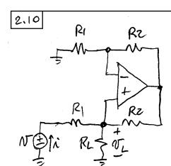
(a) Apply at the voltage V.  $V_L = R_L \dot{N}_L = R_L \frac{N}{R_I}$   $\dot{N} = \frac{V - N \dot{L}}{R_I} = \frac{1 - R_L / R_I}{R_I} V$   $R_i = N \dot{R}_i = R_I / (1 - R_L / R_I)$ . (b)  $R_L = R_I \Rightarrow V_L = R_L \frac{V}{R_I} = V \Rightarrow \dot{N} = 0$
