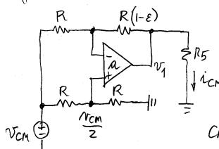
(a) A=00,  $E=4\frac{P}{100}=0.04$ . Superposition:  $V_1=-\frac{R(I-E)}{R}U_{CM}$   $+\left[1+\frac{R(I-E)}{R}\right] \frac{1}{2}V_{CM} = \frac{E}{2}V_{CM}$ ,  $I_{CM}=\frac{V_1}{R_5}=\frac{E/2}{R_5}$ . CMRR=20 log  $\frac{1/R_5}{(E/2)/R_5}=20\log 50=34dB$ .
