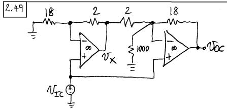
(a) Since IMSR > 18 kR > 2 kR, we expect the I-M  $\Omega$  resistor to have little effect on Adm, so  $Adm \approx 1+18/2=10$  V/V. To find Acm, the the inputs together and drive them with  $N_{TC}$ . Then, wring the superposition principle,  $N_{TC} = -\frac{18}{2}N_X + \left(1 + \frac{18}{2/1000}\right)N_{TC} = -9\left(1 + \frac{2}{18}\right)N_{TC} + \left(1 + \frac{18}{2} + \frac{18}{1000}\right)N_{TC}$
