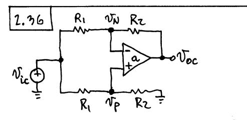
$\sqrt{SC} = A(V_P - V_N) = A \left[ \frac{Rz}{R_1 + Rz} V_{ic} - \frac{RzV_{ic} + R_1 V_{oc}}{R_1 + Rz} \right] \\
