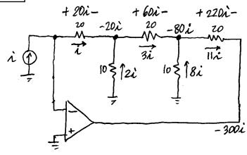
Start out a left, and work your way Toward the right via repeated application of SR, kVL, and kCl to get A=\frac{No}{iI} = -300 V/mA.
