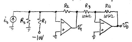
$\Delta i_{s} = (20-4) \text{ mA} = 16 \text{ mA}, \ \Delta v_{1} = -\Delta v_{0} = -8 \text{ V}, \ R_{z} = \left| \frac{\Delta V_{1}}{\Delta i_{s}} \right| = \frac{8}{16} = 500 \text{ } \Omega.$   $i_{s} = 4 \text{ mA} \Rightarrow v_{0} = 0 \Rightarrow v_{1} = 0 \Rightarrow i_{R_{z}} = 0 \Rightarrow i_{R_{1}} = i_{s} = 4 \text{ mA} \Rightarrow$   $R_{1} = 10/4 = 2.5 \text{ kg}.$
