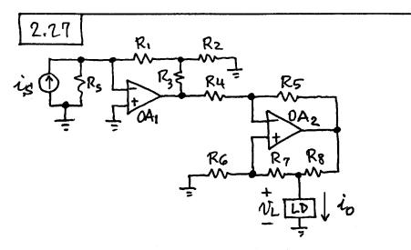
Choose the T-V converter components for a 10-V full scale at  $0A_1$ 's output. Thus, let  $R_1 = 1M\Omega$ ,  $R_2 = 1k\Omega$ ,  $R_3 = 100 k\Omega$ . io(mex) =  $10^5 \times 100 \times 10^{-9} = 10 \text{mA}$ . Disposing  $R_8 = 500 \text{ Tr}$  yields a voltage compliance of  $10-0.5 \times 10 = 5 \text{ V}$ . Finally, let  $R_4 = R_5 = R_6 = 100 \text{ kR}$ ,  $R_7 = 99.5 \text{ kD}$ .
