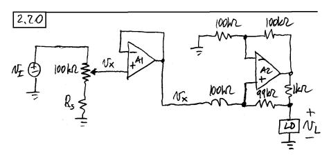
Use variable input attenuator to implement  $0.(V_{L} \leq U_{X} \leq V_{L})$ , and then use follower  $A_{1}$  to buffer  $V_{X}$  to the Howland pump with zero resistance to avoid disturbing the resistance ratios. Wiper down  $\geqslant 0.1 = R_{S}/(100 + R_{S}) \Rightarrow R_{S} = 11.1 \text{ kr. } i_{O} = \frac{V_{X}}{1 \text{ kr.}}$
