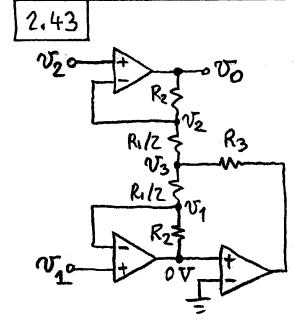
$$V_{1} = \frac{R_{2}}{R_{2} + R_{1}/2} V_{3} \Rightarrow V_{3} = \left(1 + \frac{R_{1}}{2R_{2}}\right) V_{1};$$
