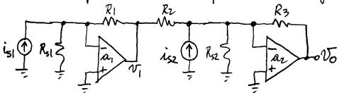
$N_0 = -R_3 \dot{n}_{S2} - \frac{R_3}{R_2} N_1 = -R_3 \dot{n}_{S2} - \frac{R_2}{R_3} (-R_1 \dot{n}_{S1}) = A_1 \dot{n}_{S1} + A_2 \dot{n}_{S2} A_2 = R_3,$   $A_1 = \frac{R_2 R_3}{R_1} \cdot A_1 = A_2 = 10 \text{ V/mA} \Rightarrow R_3 = 10 \text{ kg} \cdot \text{Need } R_2/R_1 = 1. \text{ Pick also}$   $R_1 = R_2 = 10 \text{ kg} \cdot \text{M}.$
