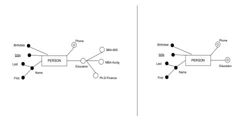
The ER diagram on the left permits specification of a maximum of three degrees - in fact, only three specific degrees. The ER diagram on the right, however, is more flexible in that it permits specification of multiple degrees of any kind including no degrees.
