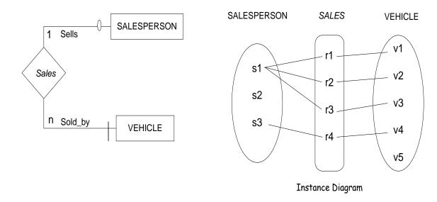
In the second ER diagram, the instance diagram on the right is not consistent with the ER diagram on the left. The ER diagram specifies total participation of SALESPERSON in relationship *Sales*. But then, s2 in the instance diagram does not participate in the relationship.
