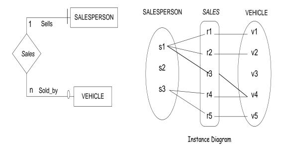
In the first ER diagram, the instance diagram on the right is not consistent with the ER diagram on the left. The ER diagram specifies total participation of VEHICLE in relationship *Sales*. But then, v3 in the instance diagram does not participate in the relationship.
