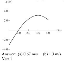
111) The graph in the figure shows the position of a particle as it travels along the *x*-axis. What is the magnitude of the instantaneous velocity of the particle when t = 1.0 s?
