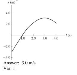
112) The graph in the figure shows the position of a particle as it travels along the *x*-axis. What is the magnitude of the average velocity of the particle between t = 1.0 s and t = 4.0 s?
