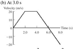
Answer: (a)  $10 \text{ m/s}^2$  (b)  $0 \text{ m/s}^2$ Var: 1 119) The figure shows a graph of the velocity of an object as a function of time. What is the average acceleration of the object over the following time intervals?
