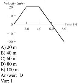
122) The figure shows a graph of the velocity of an object as a function of time. What is the displacement of the object from 0 s to 8.0 s?
