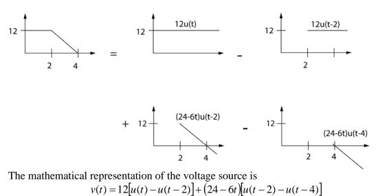
1.17 The appropriate superposition of the voltage in Figure P1.17 is illustrated below
