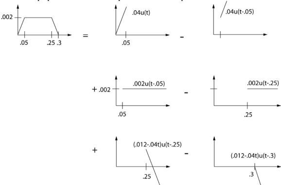
1.19 The superposition of the cam displacement over one period is shown below
