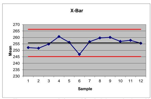
The process appears to be in control from both the  $\bar{x}$  and R charts, although sample 6 is close to the LCL and perhaps should be investigated.
