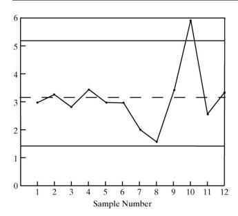
The process appears out of control for sample 10, however, this could be an aberration since there are no other apparent nonrandom patterns or out-of-control points. Thus, this point should probably be "thrown out" and a new control chart developed with the remaining eleven samples.
