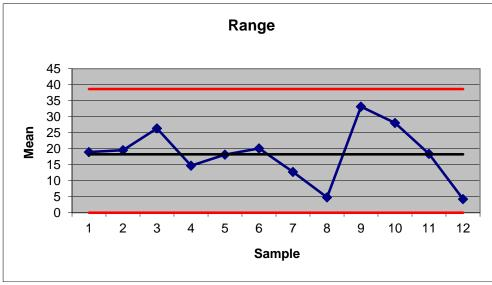
b. The process variability is within the control limits.
