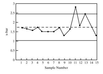
The process is not in control, thus the control chart cannot be used on a continuing basis.
