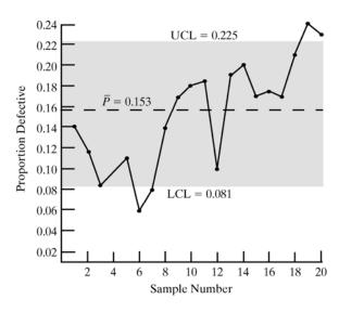
In general, the proportion of defectives increases from sample 6 to sample 20, where it is eventually above the upper control limit. This indicates the process is moving out of control.
