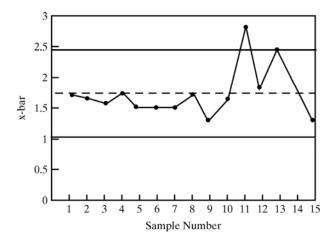
The process is not in control, thus the control chart cannot be used on a continuing basis.
