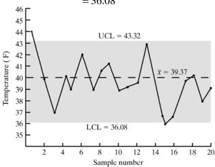
The process appears to be in control, with sample 1 seeming to be an aberration, however, the process should still be checked.
