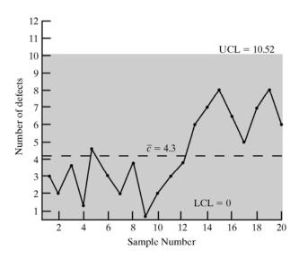
The process was not strictly out of control; however, from sample 10 to sample 20, the sample values were above the average and exhibited increasingly nonrandom behavior.
