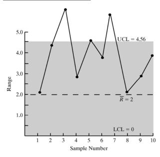
The process clearly seems to be out of control. There are three of the sample points above the UCL, and all other sample values are above the center line for  $\overline{R}$ , indicating nonrandom variations.
