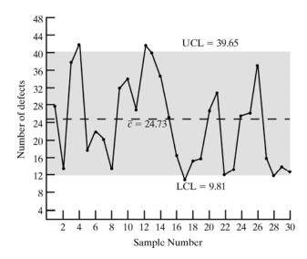
With three points outside the control limits, the process appears to be out of control.
