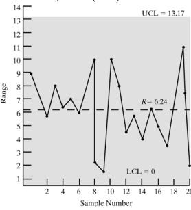
b. The temperature is within the control limits.
