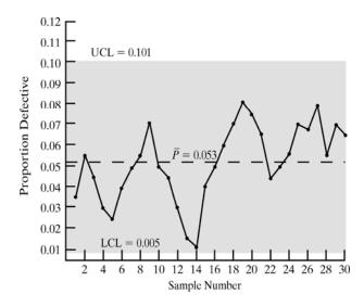
The process does not seem to be out of control.
