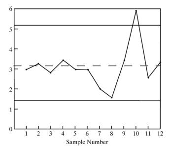
The process appears out of control for sample 10, however, this could be an aberration since there are no other apparent nonrandom patterns or out-of-control points. Thus, this point should probably be "thrown out" and a new control chart developed with the remaining eleven samples.
