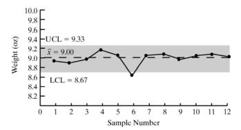
The process appears to be in control from both the  $\overline{x}$  and R charts, although sample 6 is close to the LCL and perhaps should be investigated.
