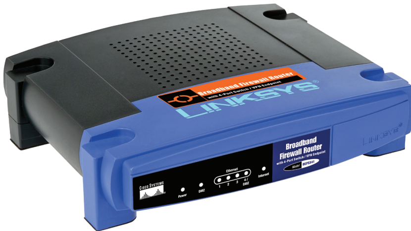
FIGURE 1-18 Linksys EtherFast® Cable/DSL Firewall Router with 4-Port Switch (courtesy of Linksys).
