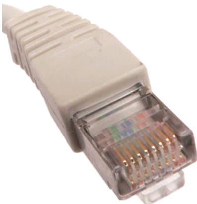
FIGURE 2-26 Wires pushed into the RJ-45 (8P8C) plug.
