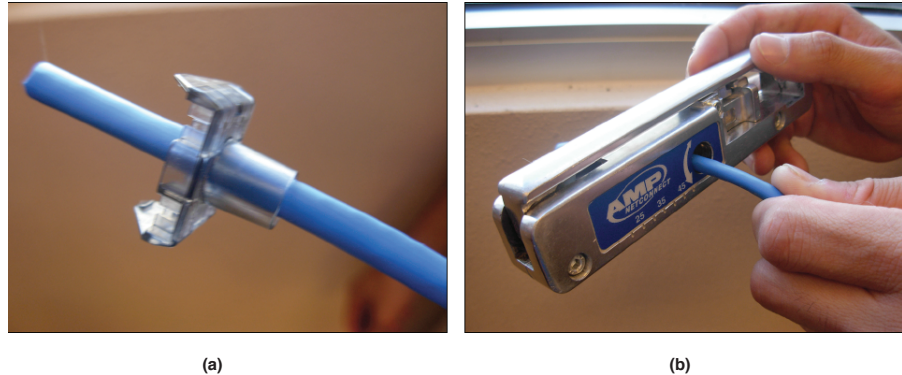
FIGURE 2-14 (a) Placing the bend-limiting strain relief boot on the cable and (b) stripping off 3 inches of jacket from the UTP cable.
