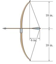
Geometry: Referring to Fig. *a*, the stretched length of the string is
