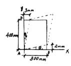
•2–13. The piece of rubber is originally rectangular and subjected to the deformation shown by the dashed lines. Determine the average normal strain along the diagonal DB and side AD.
