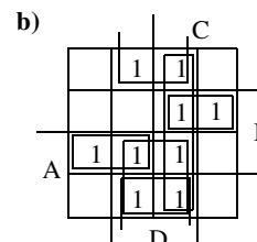
$$F = \bar{B}D + \bar{A}BC + AB\bar{C} + (AD \text{ or } CD)$$
