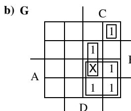
$$F = AC + \bar{A}\bar{B}\bar{C}D + \bar{A}\bar{B}\bar{C}\bar{D}$$
