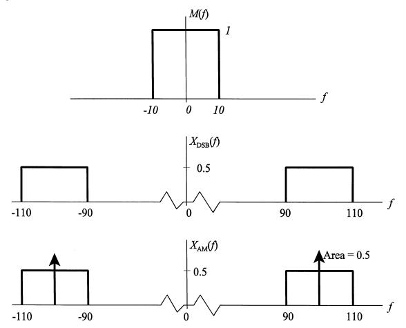
The single sideband spectra consist of the portion of the DSB spectrum from -110 to -100 and 100 to 110 Hz for USB, or the portion from -100 to -90 and from 90 to 100 for LSB.
