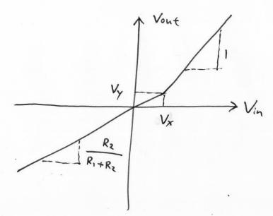
Note: at the turning point when D. starts to conduct,
