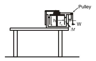
The relationship between  $\mu, r_s, \omega, h$ , and W is now developed.
