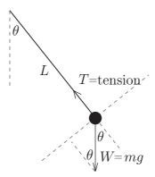
(b) The path of the particle is a circle, therefore polar coordinates are intrinsic to the problem. The variable r is radial distance and the angle  $\theta$  is measured from the vertical.
