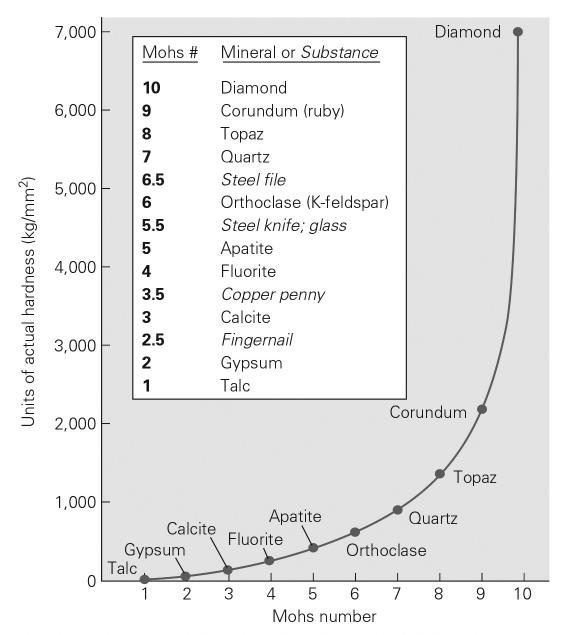
Mohs's numbers are relative—in reality, diamond is 3.5 times harder than corundum, as the graph shows.
