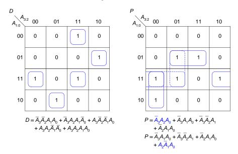
Hardware implementations are below (implementing the first minimal equation given for P).
