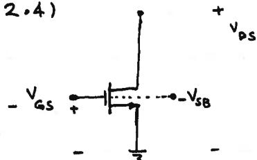
$I_D$  versus  $V_{GS}$ : (for NMOS)I) for  $V_{GS} < V_{TH}$ ,  $I_D \approx 0$ II) for  $V_{TH} < V_{GS} < V_{TH} + V_{DS}$   $\Rightarrow$  Device is in the Saturation region
