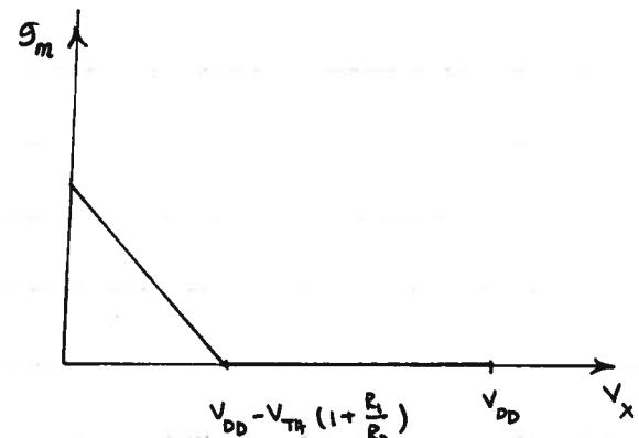
If  $V_{DD} - V_{TH} (1 + \frac{R_2}{R_1}) < 0$  device doesn't turn on.
