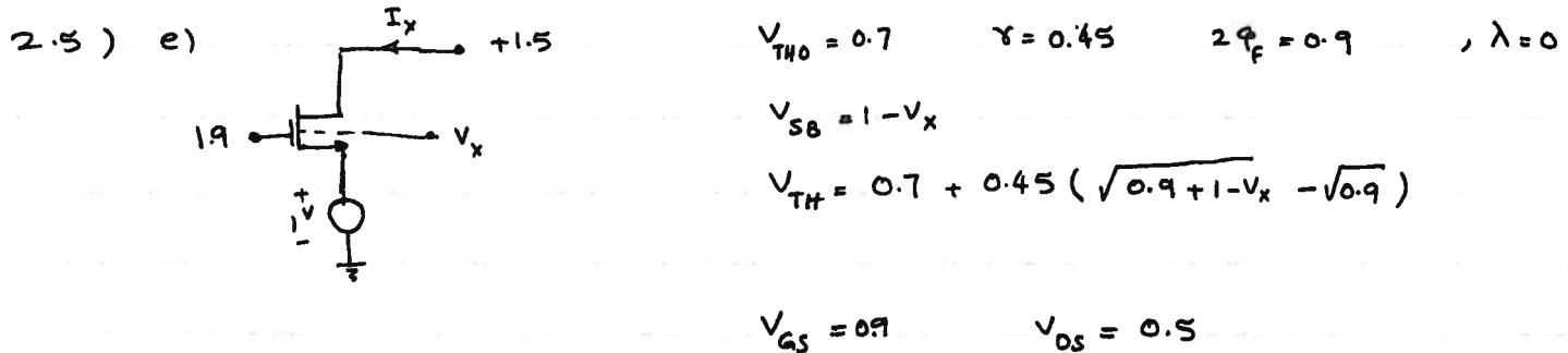
for  $V_x = 0$ ,  $V_{TH} = 0.893$  So device is in saturation region.
