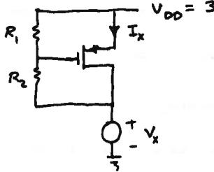
$$V_{SG} = (V_{DD} - V_X) \frac{R_1}{R_1 + R_2}$$
