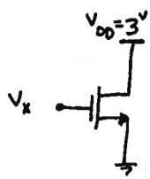
for  $V_x < V_{th} (= 0.7)$  device is off ,  $I_D \approx 0$
