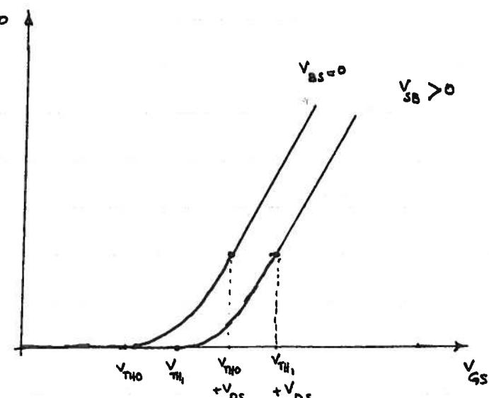
Changing  $V_{SB}$  just shifts the curve to the right for  $V_{SB} > 0$  or to the left for  $V_{SB} < 0$
