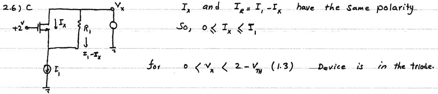
$$V_{GS} = 2 - V_x + R_1(I_1 - I_x), \quad V_{DS} = R_1(I_1 - I_x)$$
