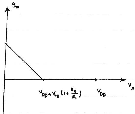
If  $V_{DD} + V_{TH} \left(1 + \frac{R_2}{R_1}\right) < 0$  (e.g. for small value of  $R_1$ ), device never turns on!
