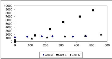
Cost A varies in total amount, but the variation does not appear to be related to variation in volume of the cost driver. In addition, total cost is fairly high when volume of the cost driver is zero. It is most likely a fixed cost.
