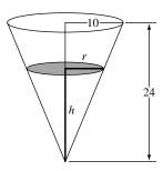
**26.** Find  $\frac{dh}{dt}\Big|_{h=6}$  given that  $\frac{dV}{dt} = 8$ .  $V = \frac{1}{3}\pi r^2 h$ , but  $r = \frac{1}{2}h$  so  $V = \frac{1}{3}\pi \left(\frac{h}{2}\right)^2 h = \frac{1}{12}\pi h^3$ ,  $\frac{dV}{dt} = \frac{1}{4}\pi h^2 \frac{dh}{dt}$ ,  $\frac{dh}{dt} = \frac{4}{\pi h^2} \frac{dV}{dt}$ ,  $\frac{dh}{dt}\Big|_{h=6} = \frac{4}{\pi (6)^2} (8) = \frac{8}{9\pi}$  ft/min.
