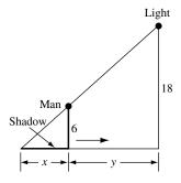
(b) The tip of the shadow is z = x + y feet from the street light, thus the rate at which it is moving is given by  $\frac{dz}{dt} = \frac{dx}{dt} + \frac{dy}{dt}$ . In part (a) we found that  $\frac{dx}{dt} = -\frac{3}{2}$  when  $\frac{dy}{dt} = -3$  so  $\frac{dz}{dt} = (-3/2) + (-3) = -9/2$  ft/s; the tip
